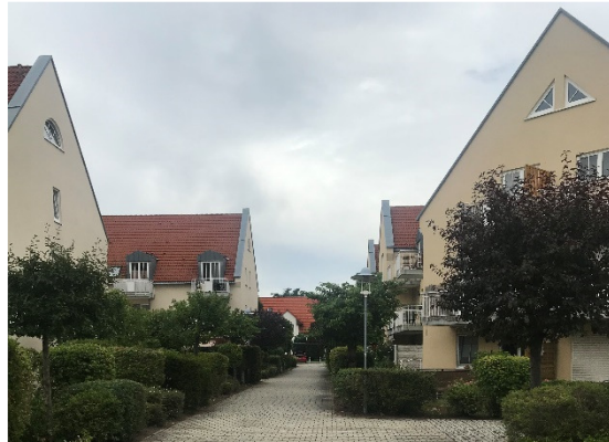
This development in Coswig, Germany has a wide shared path for pedestrians and cyclists at its heart. Access and parking for vehicles is pushed to the perimeter of the development to help create a comfortable pedestrian environment. Pedestrians and cyclists can share this route due to it being sufficiently wide.
